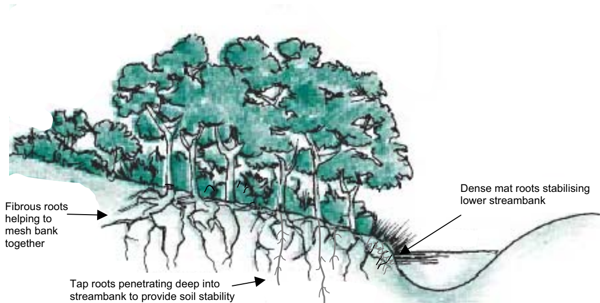
Cross section of a stream showing the matrix of tap and fibrous roots from different species acting to stabilise the streambank (Diagram modified after Price & Lovett 2002)
